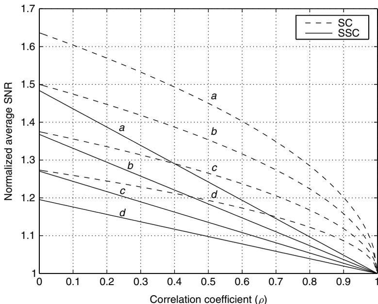
**Figure 9.40.** Comparison of the normalized average SNR of SC ( $\bar{\gamma}_{SC}/\bar{\gamma}$ ) and SSC ( $\bar{\gamma}_{SSC}/\bar{\gamma}$ ) versus correlation coefficients( $\rho$ ) over Nakagami fading with parameter (a)  $m = 0.5$ , (b)  $m = 1$ , (c)  $m = 2$ , and (d)  $m = 4$ .
