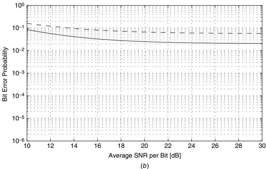
**Figure 12.10.** TUB (solid line) and union–Chernoff (dashed line) bound on average BEP performance of differential detection with unknown CSI in fast Rayleigh fading: land-mobile channel: (a)  $f_d T_b = 0.05$ ; (b)  $f_d T_b = 0.1$ .
