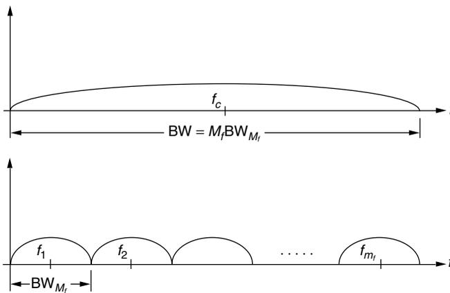
**Figure 11.1.** Comparison between single and multicarrier DS-CDMA systems power spectral densities.
