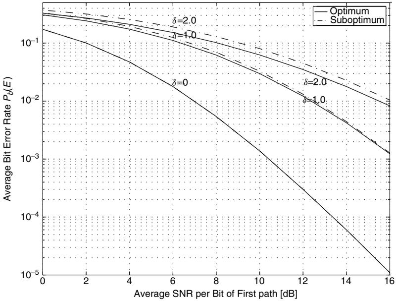
**Figure 7.8.** Comparison of the average BEP performance for optimum and suboptimum reception of noncoherently detected binary FSK over Rayleigh fading with an exponential PDP;  $L_p = 4$ , varying  $\delta$ ,  $m = 1$ ,  $M = 2$ .
