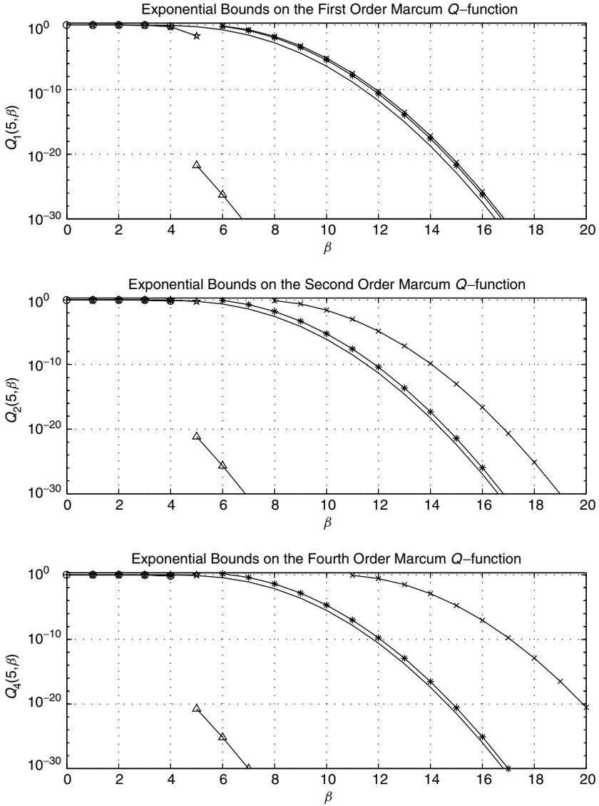
**Figure 4.3.** Plots of  $Q_1(5, \beta)$ ,  $Q_2(5, \beta)$ ,  $Q_4(5, \beta)$ , and their bounds versus  $\beta$ . —, Exact; \*, upper bound of (4.57a); x, Chernoff upper bound from Ref. 23; ☆, Chernoff lower bound from Ref. 23; Δ, lower bound of (4.62).
