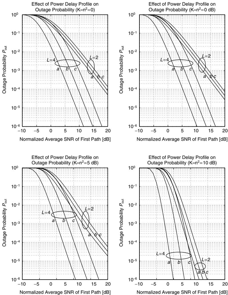
**Figure 9.14.** Outage probability with MRC or postdetection EGC reception ( $L = 2$  and  $4$ ) versus normalized average SNR of the first path  $\bar{\gamma}_1/\gamma_{th}$  over a Rician fading channel with an exponentially decaying power delay profile: (a)  $\delta = 0$ ; (b)  $\delta = 0.5$ ; (c)  $\delta = 1$ .
