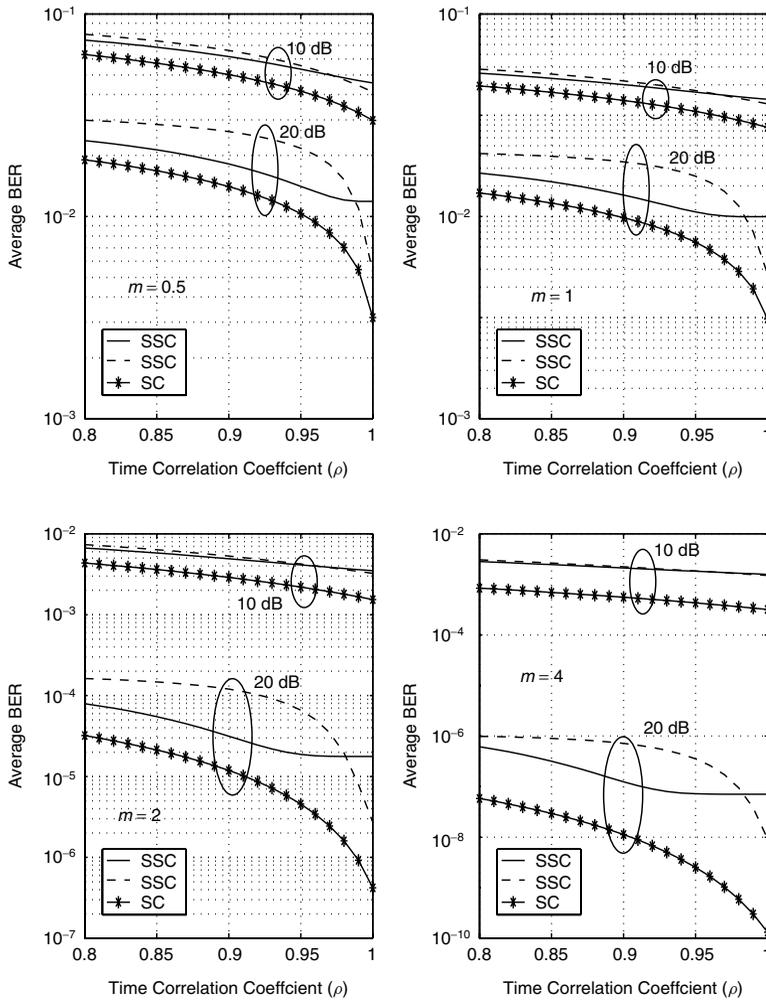
**Figure 9.45.** Average BER of binary DPSK with SC and SSC versus correlation coefficient ( $\rho$ ) with  $\bar{\gamma} = 10$  dB and  $\bar{\gamma} = 20$  dB. The dashed line corresponds to the case where the optimum threshold is set for  $\rho = 1$  or equivalently  $\tau = 0$ . The solid line corresponds to the case where the optimum threshold is optimized over  $\rho = 0.8$  to 1 range.
