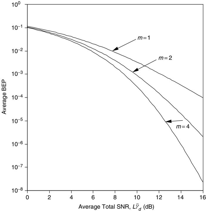
**Figure 10.7.** Average BEP of the optimum combiner in Nakagami- $m$  fading with a single fading co-channel interferer;  $\bar{\gamma}_d = \bar{\gamma}_l$ ,  $L = 4$ .
