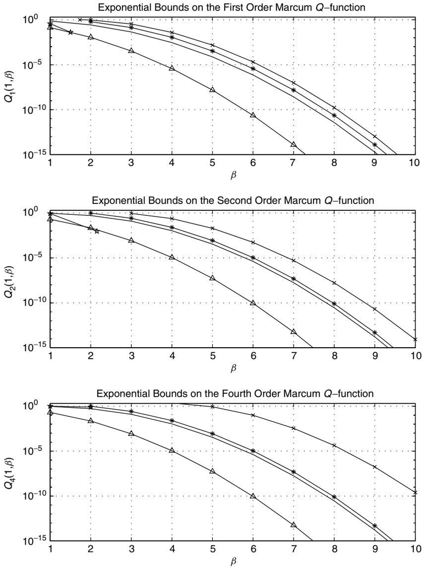
**Figure 4.2.** Plots of  $Q_1(1, \beta)$ ,  $Q_2(1, \beta)$ ,  $Q_4(1, \beta)$ , and their bounds versus  $\beta$ : —, Exact; \*, upper bound (4.57a); ×, Chernoff upper bound from Ref. 23; ☆, Chernoff lower bound from Ref. 23; △, lower bound of (4.62).
