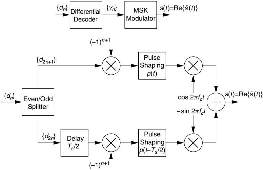
Figure 3.11. Equivalent real forms of precoded MSK transmitters.
