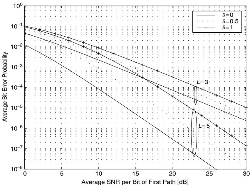
**Figure 9.3.** Average BER of BPSK with  $L$ -fold MRC diversity versus the SNR per bit of the first path for an  $L$ -path frequency-selective Nakagami- $m$  ( $m = 0.5$ ) fading channel with an exponentially decaying power delay profile.  $\delta$  is the power decay factor.
