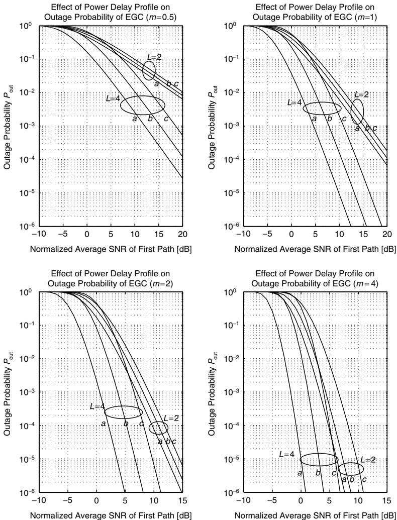
**Figure 9.15.** Outage probability with EGC reception ( $L = 2$  and  $4$ ) versus normalized average SNR of the first path  $\bar{\gamma}_1 / \gamma_{th}$  over a Nakagami- $m$  fading channel with an exponentially decaying power delay profile: (a)  $\delta = 0$ ; (b)  $\delta = 0.5$ ; (c)  $\delta = 1$ .
