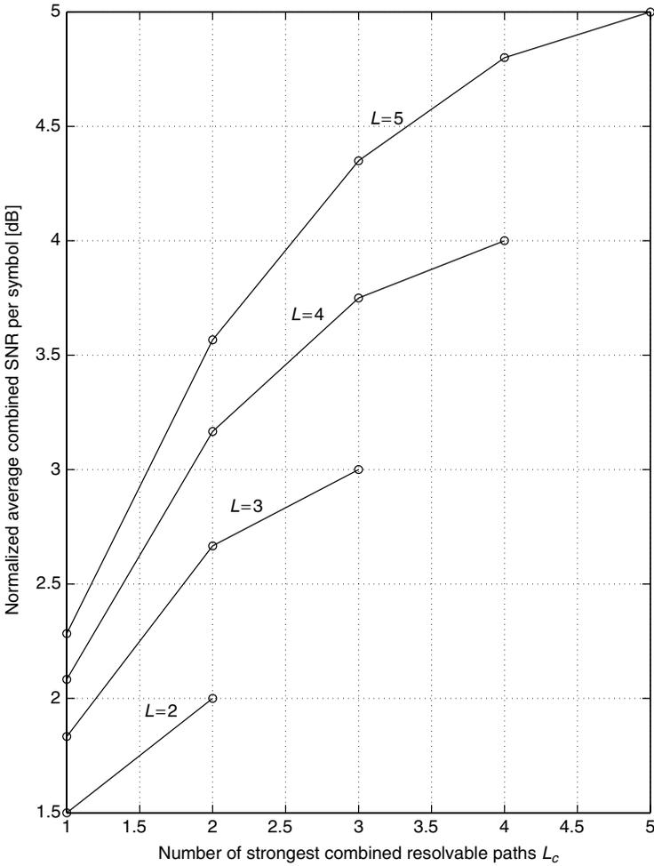
**Figure 9.47.** Normalized average combined SNR  $\bar{\gamma}_{\text{GSC}}/\bar{\gamma}$  versus the number of the strongest combined paths  $L_c$  for various values of the number of the resolvable paths  $L$ .
