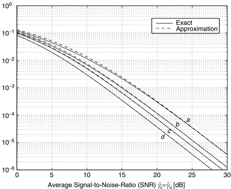
**Figure 9.25.** Exact and approximate average BER of BPSK versus average SNR of the first branch for equal average branch SNRs ( $\bar{\gamma}_1 = \bar{\gamma}_2$ ) and for various values of the correlation coefficient: (a)  $\rho = 0.9$ ; (b)  $\rho = 0.7$ ; (c)  $\rho = 0.5$ ; (d)  $\rho = 0$ .
