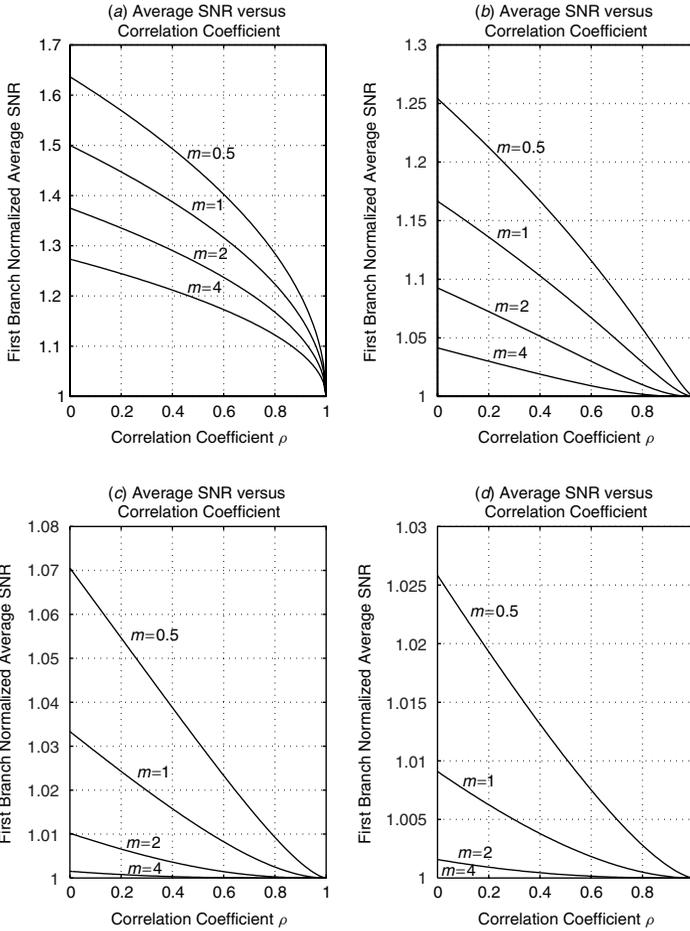
**Figure 9.23.** First branch normalized average SNR ( $\bar{\gamma}_{sc}/\bar{\gamma}_1$ ) of SC versus correlation coefficient ( $\rho$ ) for correlated Nakagami- $m$  fading channels with (a)  $\bar{\gamma}_1 = \bar{\gamma}_2$ , (b)  $\bar{\gamma}_1 = 2\bar{\gamma}_2$ , (c)  $\bar{\gamma}_1 = 5\bar{\gamma}_2$ , and (d)  $\bar{\gamma}_1 = 10\bar{\gamma}_2$ .
