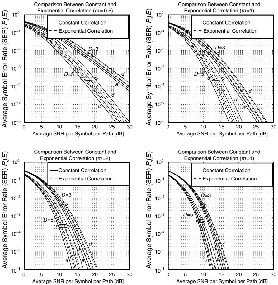
**Figure 9.18.** Comparison of the average SER of 16-QAM with MRC diversity for constant and exponential fading correlation profiles and various values of the correlation coefficient: (a)  $\rho = 0$ ; (b)  $\rho = 0.2$ ; (c)  $\rho = 0.4$ ; (d)  $\rho = 0.6$ .  $\bar{\gamma}_d = \bar{\gamma}$  for  $d = 1, 2, \dots, D$ .
