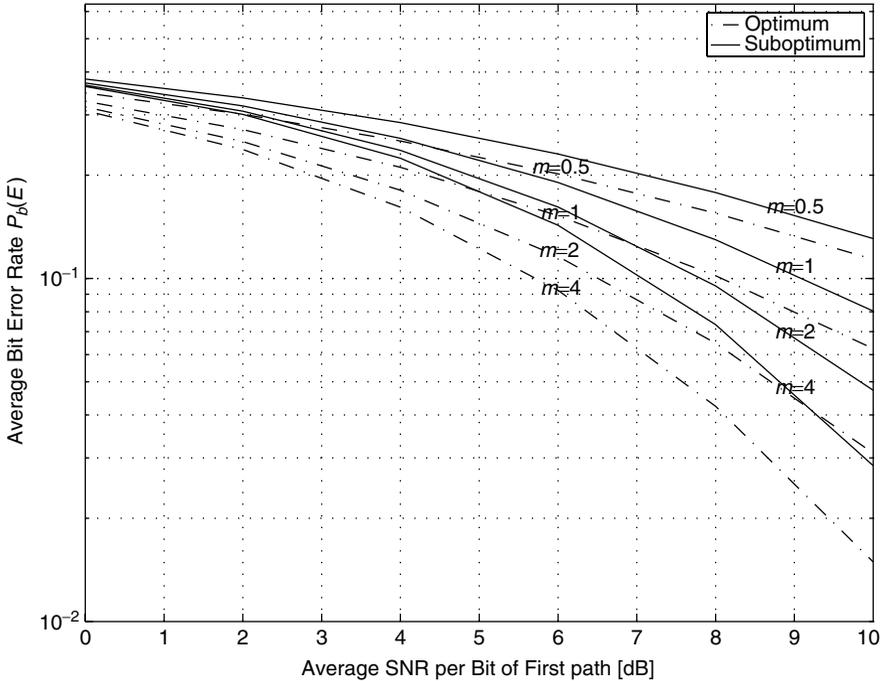
**Figure 7.10.** Comparison of the average BEP performance for optimum and suboptimum reception of noncoherently detected binary FSK over Nakagami- $m$  fading with an exponential PDP;  $\delta = 2.0$ ,  $L_p = 4$ , varying  $m$ .
