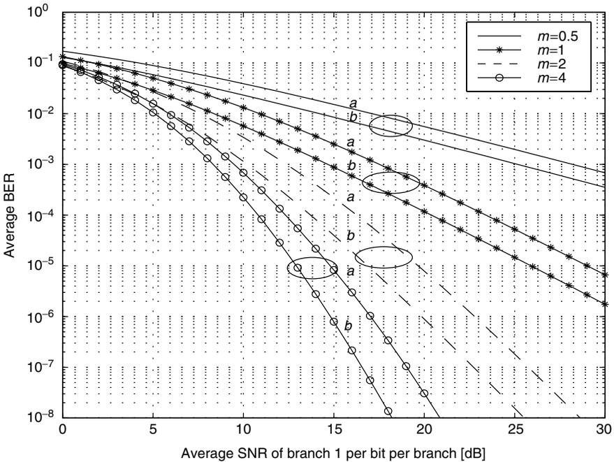
**Figure 9.39.** Average BER of BPSK versus average SNR of the first branch  $\bar{\gamma}_1$  (a) for unequal average branch SNRs  $\bar{\gamma}_1 = \bar{\gamma}_2/5$  and (b) for equal average branch SNRs  $\bar{\gamma}_1 = \bar{\gamma}_2$  over Nakagami- $m$  fading channels.
