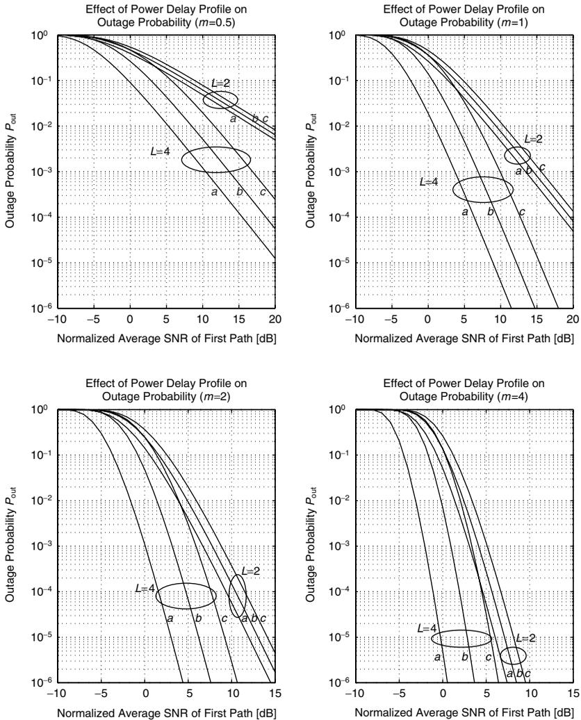
**Figure 9.13.** Outage probability with MRC or postdetection EGC RAKE reception ( $L = 2$  and 4) versus normalized average SNR of the first path  $\bar{\gamma}_1/\gamma_{th}$  over a Nakagami- $m$  fading channel with an exponentially decaying power delay profile: (a)  $\delta = 0$ ; (b)  $\delta = 0.5$ ; (c)  $\delta = 1$ .
