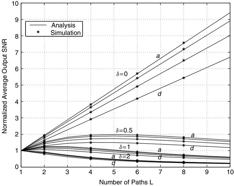
**Figure 9.4.** Normalized average output SNR  $\bar{\gamma}_{\text{EGC}}/\bar{\gamma}_1$  of coherent EGC over Nakagami- $m$  channels with an exponentially decaying power delay profile: (a)  $m = 4$ ; (b)  $m = 2$ ; (c)  $m = 1$ ; (d)  $m = 0.5$ .
