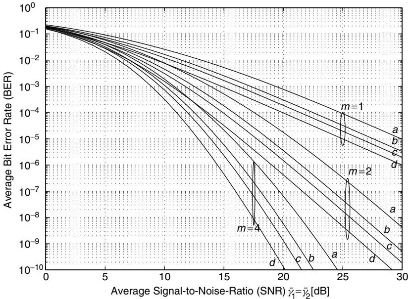
**Figure 9.26.** Average BER of BDPSK versus average SNR of the first branch for equal average branch SNRs ( $\bar{\gamma}_1 = \bar{\gamma}_2$ ) and for various values of the correlation coefficient: (a)  $\rho = 0.9$ ; (b)  $\rho = 0.7$ ; (c)  $\rho = 0.5$ ; (d)  $\rho = 0$ .
