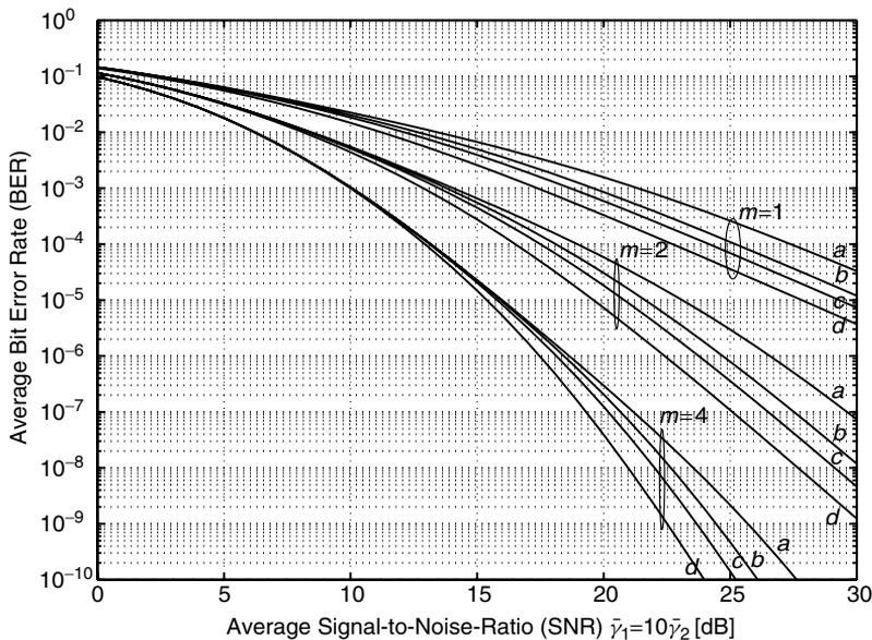
**Figure 9.29.** Average BER of BPSK versus average SNR of the first branch for unequal average branch SNRs ( $\bar{\gamma}_1 = 10\bar{\gamma}_2$ ) and for various values of the correlation coefficient: (a)  $\rho = 0.9$ ; (b)  $\rho = 0.7$ ; (c)  $\rho = 0.5$ ; (d)  $\rho = 0$ .
