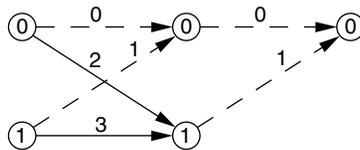
Figure 12.4. Trellis diagram and QPSK signal assignment.
