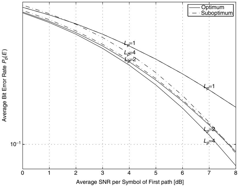
**Figure 7.9.** Comparison of the average BEP performance for optimum and suboptimum reception of noncoherently detected 4-ary FSK over Rayleigh fading with an exponential PDP;  $\delta = 1.0$ , varying  $L_p$ ,  $m = 1$ ,  $M = 4$ .
