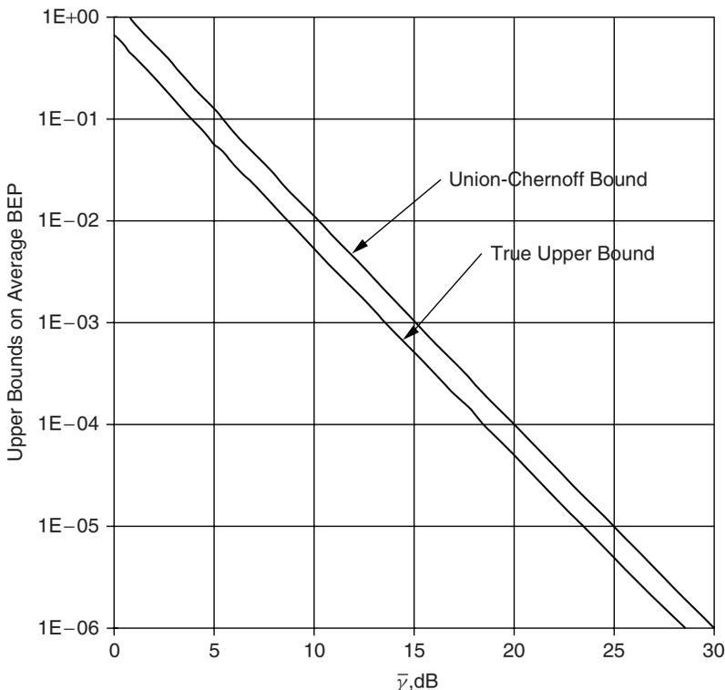
**Figure 12.7.** Upper bounds on the average bit error probability for rate  $-\frac{1}{2}$  trellis-coded QPSK with two-state trellis: coherent detection with known channel state information, Rayleigh fading.
