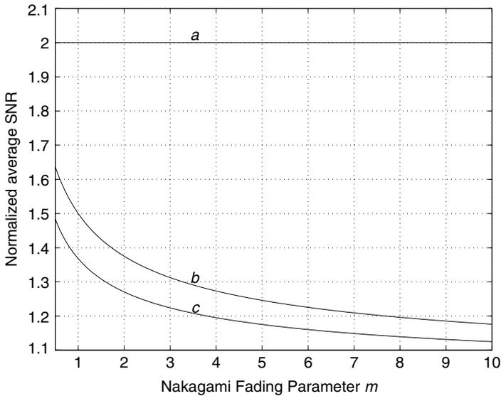
**Figure 9.32.** Normalized average SNR of (a) MRC  $(\bar{\gamma}_{MRC}/\bar{\gamma})$ , (b) SC  $(\bar{\gamma}_{SC}/\bar{\gamma})$ , and (c) SSC  $(\bar{\gamma}_{SSC}/\bar{\gamma})$  versus the Nakagami- $m$  fading parameter  $m$ .
