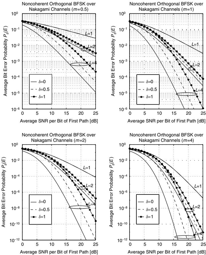
**Figure 9.10.** Average bit error probability  $P_b(E)$  of binary FSK with square-law combining versus the average SNR per bit of the first path  $\bar{\gamma}_1$  over Nakagami- $m$  channels with an exponentially decaying power delay profile.
