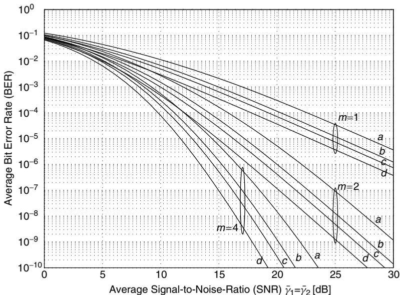
**Figure 9.28.** Average BER of BPSK versus average SNR of the first branch for equal average branch SNRs ( $\bar{\gamma}_1 = \bar{\gamma}_2$ ) and for various values of the correlation coefficient: (a)  $\rho = 0.9$ ; (b)  $\rho = 0.7$ ; (c)  $\rho = 0.5$ ; (d)  $\rho = 0$ .
