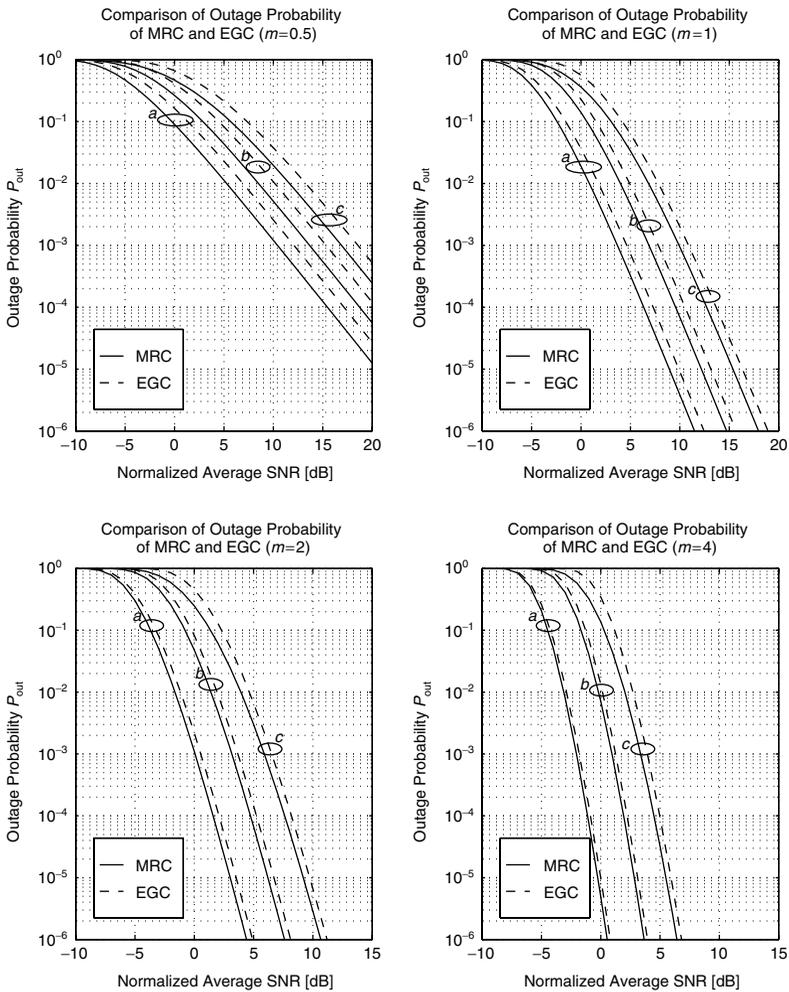
**Figure 9.16.** Comparison of the outage probability of MRC and EGC ( $L = 4$ ) versus normalized average SNR of the first path  $\bar{\gamma}_1/\gamma_{th}$  over a Nakagami- $m$  fading channel with an exponentially decaying power delay profile: (a)  $\delta = 0$ ; (b)  $\delta = 0.5$ ; (c)  $\delta = 1$ .
