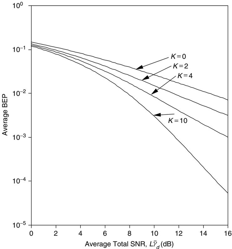
**Figure 10.4.** Average BEP of the optimum combiner in Rician fading with a single fading co-channel interferer;  $\bar{\gamma}_d = \bar{\gamma}_I$ ,  $L = 2$ .
