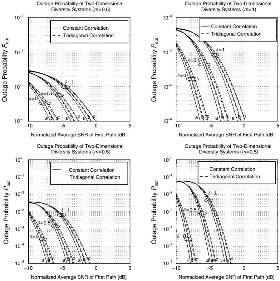
**Figure 9.64.** Outage probability with two-dimensional MRC or postdetection EGC RAKE reception ( $L_c = 4$  and  $D = 3$ ) over an exponentially decaying PDP and constant or tridiagonal spatial correlation between the antennas for various values of the correlation coefficient: (a)  $\rho = 0$ ; (b)  $\rho = 0.2$ ; (c)  $\rho = 0.4$ .
