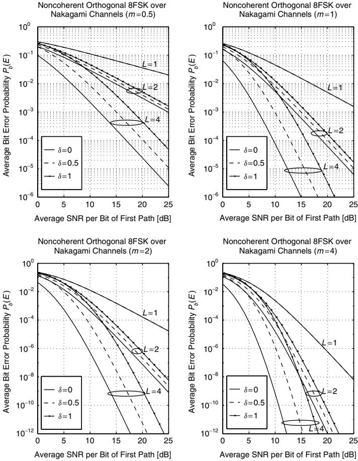
**Figure 9.12.** Average bit error probability  $P_b(E)$  of 8-ary FSK with square-law combining versus the average SNR per bit of the first path  $\bar{\gamma}_1/3$  over Nakagami- $m$  channels with an exponentially decaying power delay profile.
