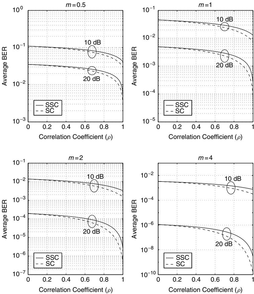
**Figure 9.44.** Average BER of binary DPSK with SC and SSC versus correlation coefficient ( $\rho$ ) with  $\bar{\gamma} = 10$  dB and  $\bar{\gamma} = 20$  dB over Nakagami- $m$  fading channel. The optimum threshold is set according to (9.308) and is thus a function of  $\rho$  and  $\bar{\gamma}$ .
