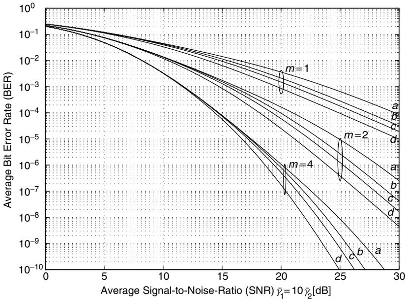
**Figure 9.27.** Average BER of BDPSK versus average SNR of the first branch for unequal average branch SNRs ( $\bar{\gamma}_1 = 10\bar{\gamma}_2$ ) and for various values of the correlation coefficient: (a)  $\rho = 0.9$ ; (b)  $\rho = 0.7$ ; (c)  $\rho = 0.5$ ; (d)  $\rho = 0$ .
