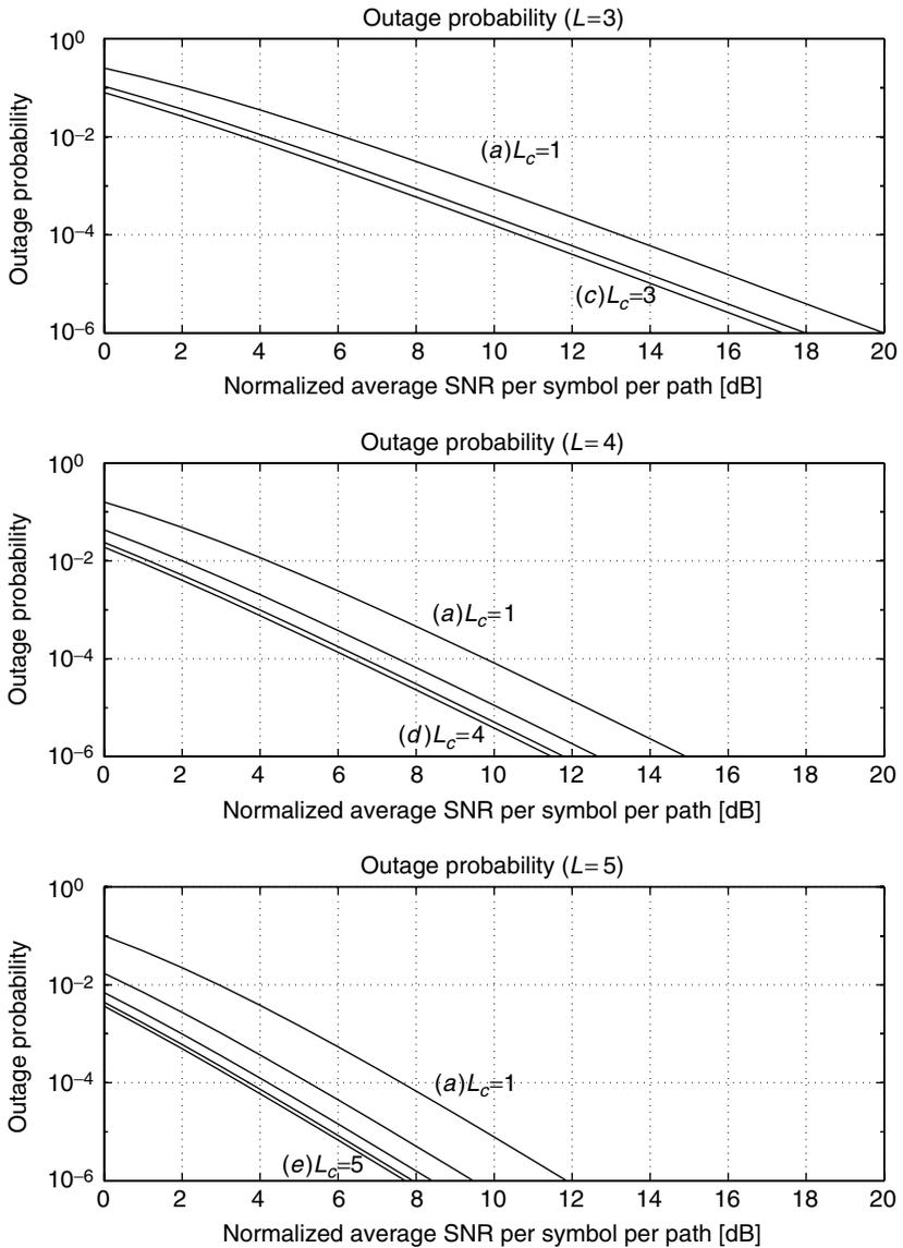
**Figure 9.48.** Outage probability  $P_{\text{out}}^{\text{GSC}}$  versus the normalized average SNR per path  $\bar{\gamma}/\gamma_{\text{th}}$ .
