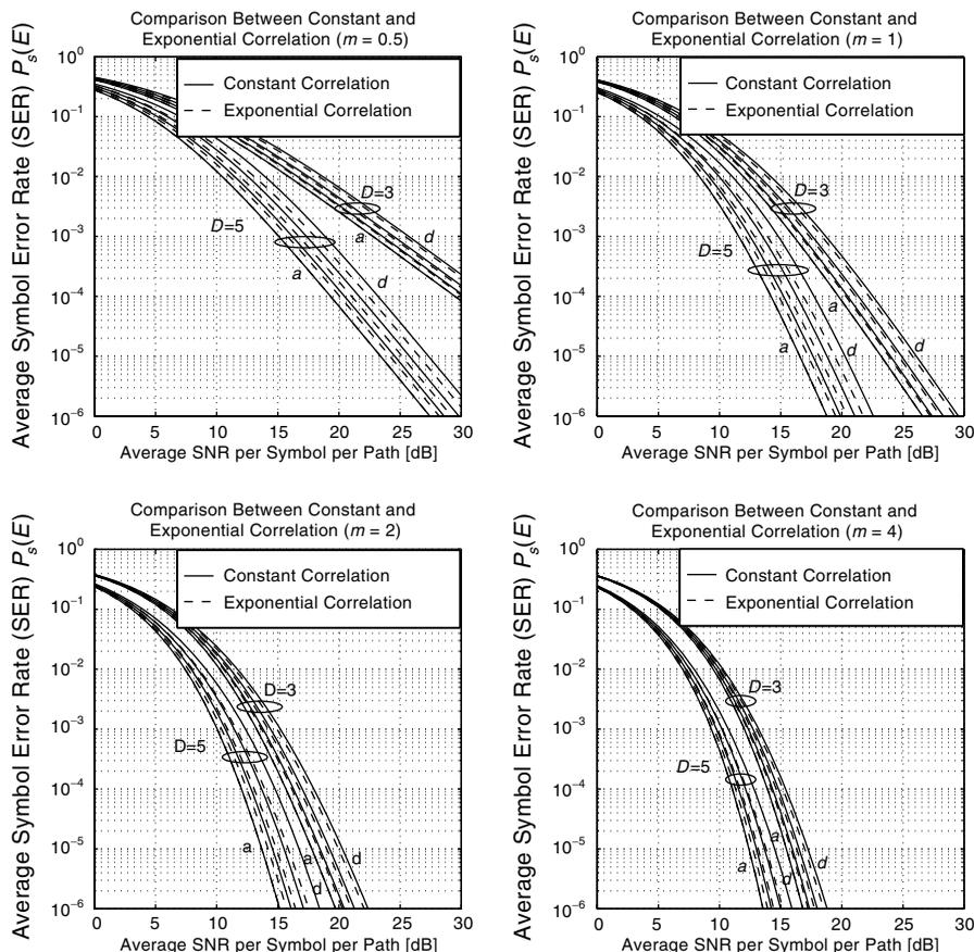
**Figure 9.17.** Comparison of the average SER of 8-PSK with MRC diversity for constant and exponential fading correlation profiles and various values of the correlation coefficient: (a)  $\rho = 0$ ; (b)  $\rho = 0.2$ ; (c)  $\rho = 0.4$ ; (d)  $\rho = 0.6$ .  $\bar{\gamma}_d = \bar{\gamma}$  for  $d = 1, 2, \dots, D$ .
