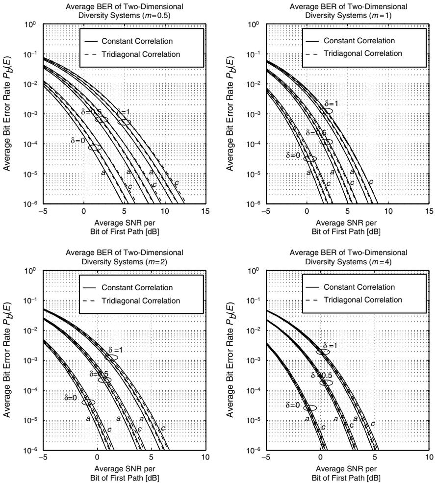
**Figure 9.63.** Average BER of BPSK with two-dimensional MRC RAKE reception ( $L_c = 4$  and  $D = 3$ ) over an exponentially decaying power delay profile and constant or tridiagonal spatial correlation between the antennas for various values of the correlation coefficient: (a)  $\rho = 0$ ; (b)  $\rho = 0.2$ ; (c)  $\rho = 0.4$ .
