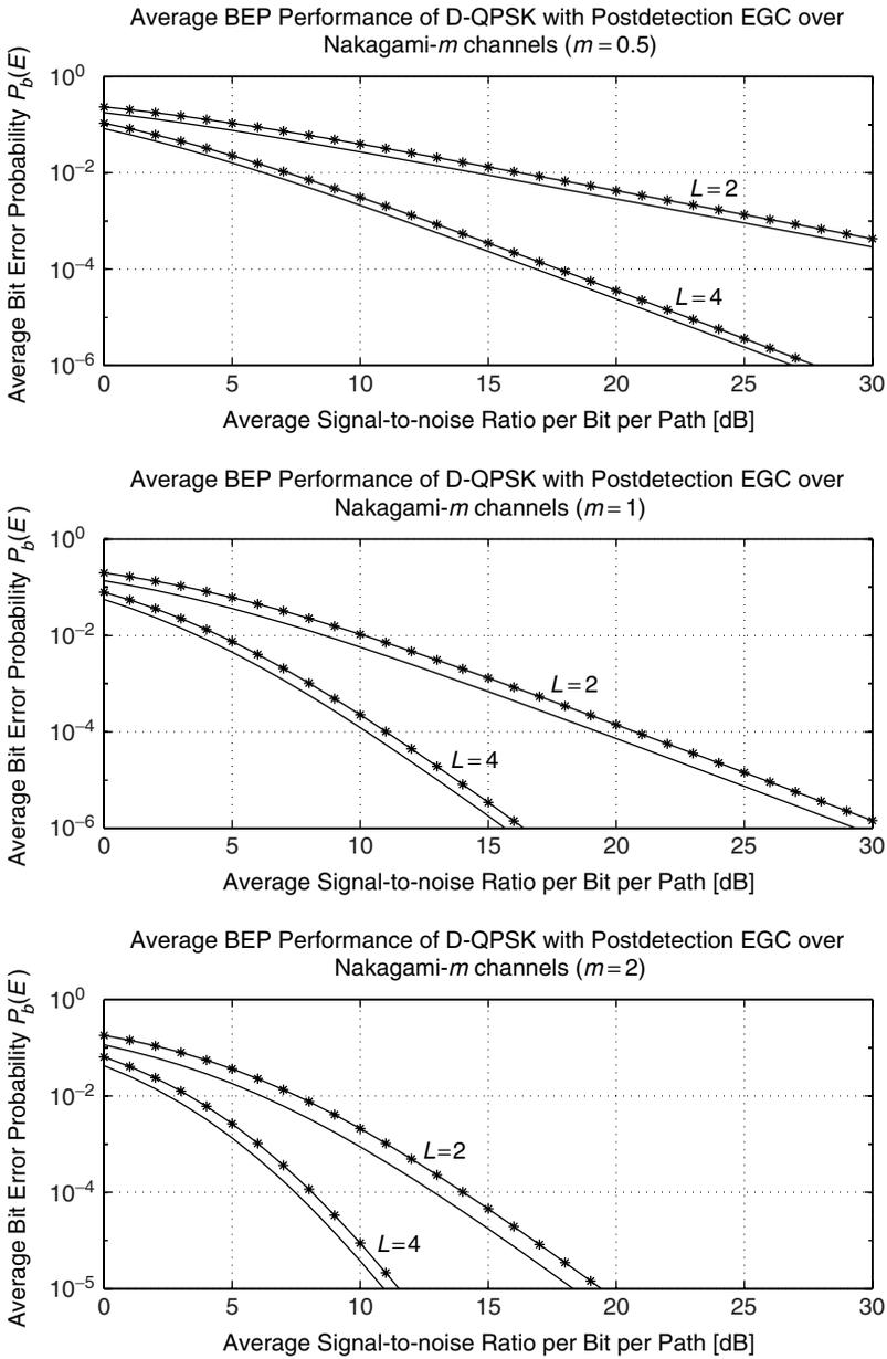
**Figure 9.9.** Average bit error probability of D-QPSK with  $L$ -fold diversity postdetection EGC versus the average SNR per bit per path for various Nakagami- $m$  fading channels. The fading is assumed to be identically distributed over the  $L$  combined paths.
