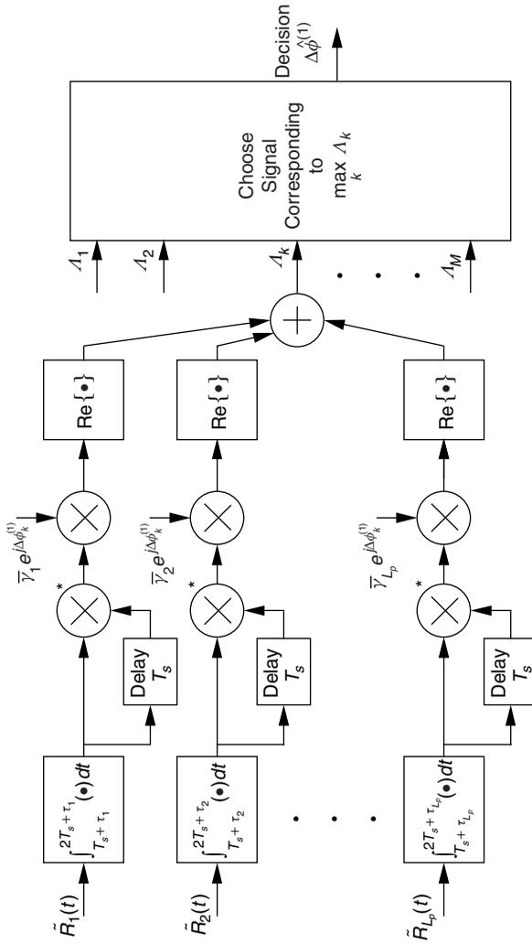
**Figure 7.11.** Complex form of optimum receiver for known phases, unknown amplitudes and delays: Rayleigh fading, two-symbol observation (conventional differentially coherent detection).
