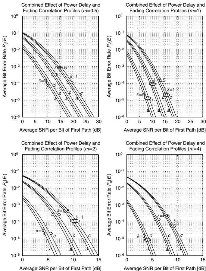
**Figure 9.19.** Average BER of BPSK with MRC reception ( $D = 5$ ) over an exponentially decaying power delay profile and an exponential correlation profile across the multipaths for various values of the correlation coefficient: (a)  $\rho = 0$ ; (b)  $\rho = 0.2$ ; (c)  $\rho = 0.4$ .
