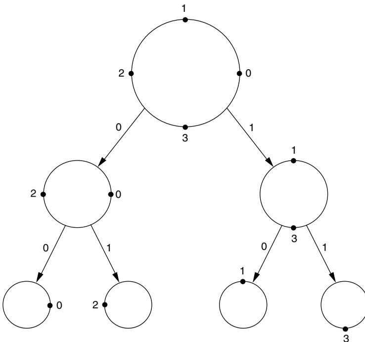
Figure 12.3. Set partitioning of QPSK signal constellation.
