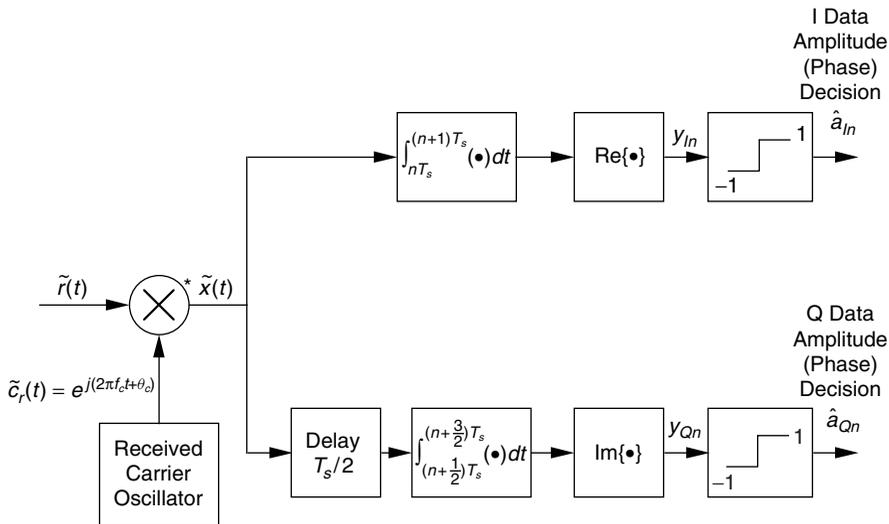
**Figure 3.7.** Complex form of optimum receiver for ideal coherent detection of OQPSK over the AWGN.
