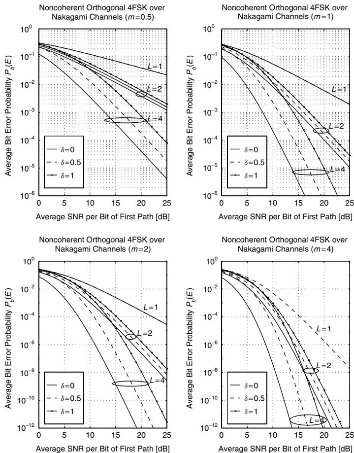
**Figure 9.11.** Average bit error probability  $P_b(E)$  of 4-ary FSK with square-law combining versus the average SNR per bit of the first path  $\bar{\gamma}_1/2$  over Nakagami- $m$  channels with an exponentially decaying power delay profile.
