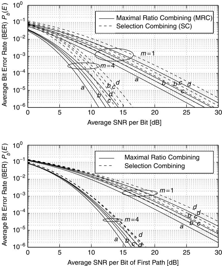
**Figure 9.30.** Comparison of average BER of BPSK with MRC and SC for various values of the correlation coefficient: (a)  $\rho = 0$ ; (b)  $\rho = 0.5$ ; (c)  $\rho = 0.7$ ; (d)  $\rho = 0.9$ . (Top) equal average branch SNRs ( $\bar{\gamma}_1 = \bar{\gamma}_2$ ); (bottom) unequal average branch SNRs ( $\bar{\gamma}_1 = 10\bar{\gamma}_2$ ).
