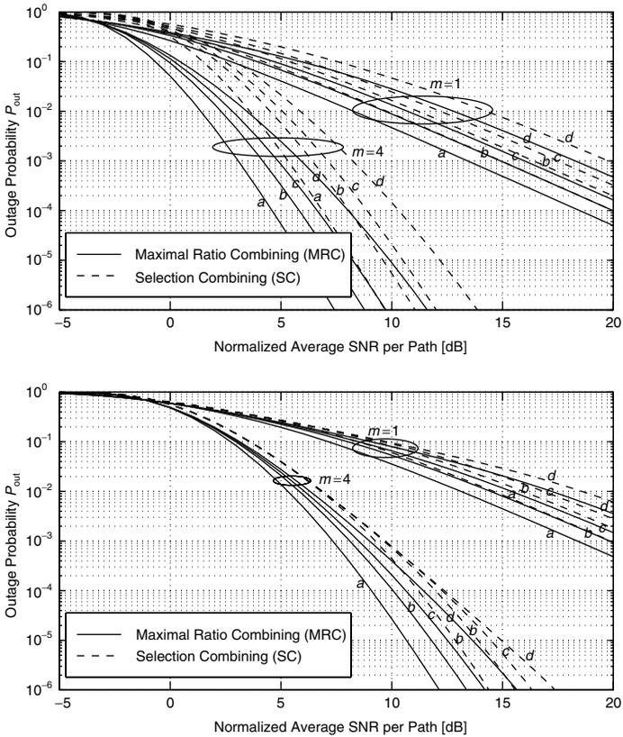
**Figure 9.24.** Comparison of outage probability with MRC and SC versus average SNR of the first branch for various values of the correlation coefficient: (a)  $\rho = 0$ ; (b)  $\rho = 0.5$ ; (c)  $\rho = 0.7$ ; (d)  $\rho = 0.9$ . (Top) equal average branch SNRs ( $\bar{\gamma}_1 = \bar{\gamma}_2$ ); (bottom) unequal average branch SNRs ( $\bar{\gamma}_1 = 10\bar{\gamma}_2$ ).
